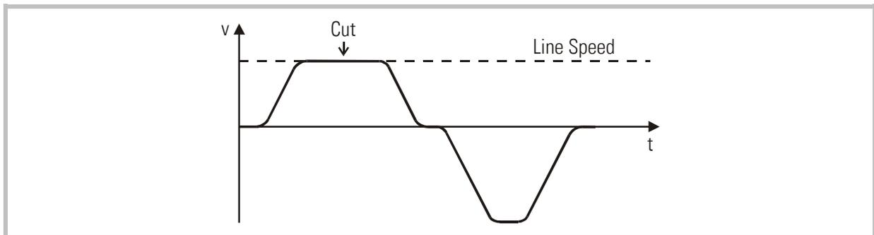
The FS340 or FS641 controller continuously measures the line speed and calculates an anticipation value to start the carriage before the cutting length is reached. Thus the shear will exactly match the cutting position of the material upon completion of the acceleration ramp and no overshoot or oscillation will take place prior to the cut. This saves time and increases the cutting efficiency of the shear system considerably.
